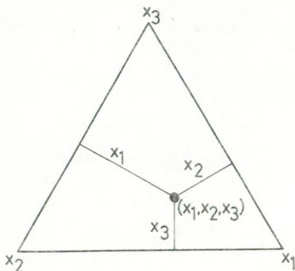
Fig. 5 Determination of  $(x_1, x_2, x_3)$  by perpendicular projection.
