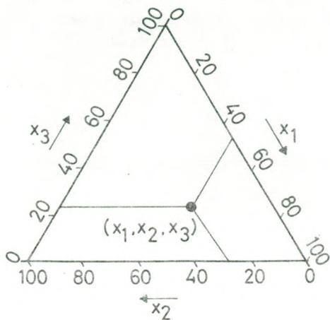
Fig. 3 Determination of coordinates of  $(x_1, x_2, x_3)$  by parallel projection.
