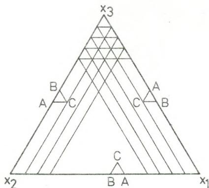
Fig. 7 Subdivision of experimental space for a three-component mixture.
