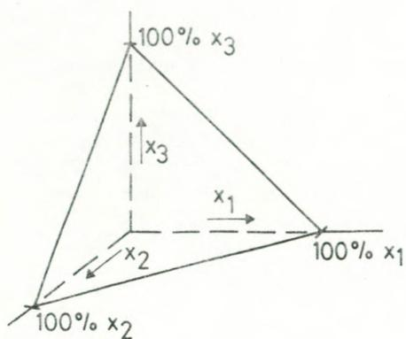
Fig. 1 The experimental space of a three-component mixture.
