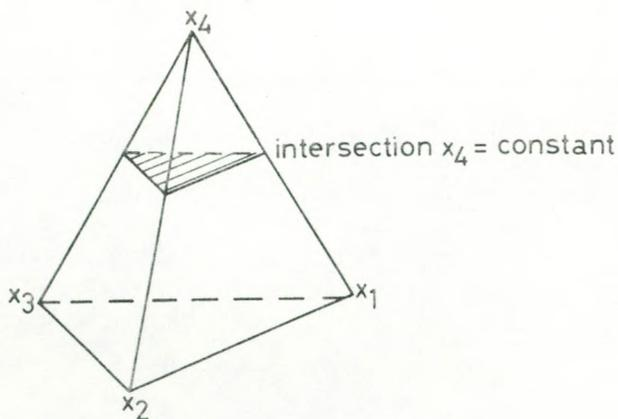
Fig. 6 Representation of experimental space in a four-component mixture.
